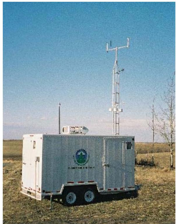
Portable Continuous Monitoring Station
